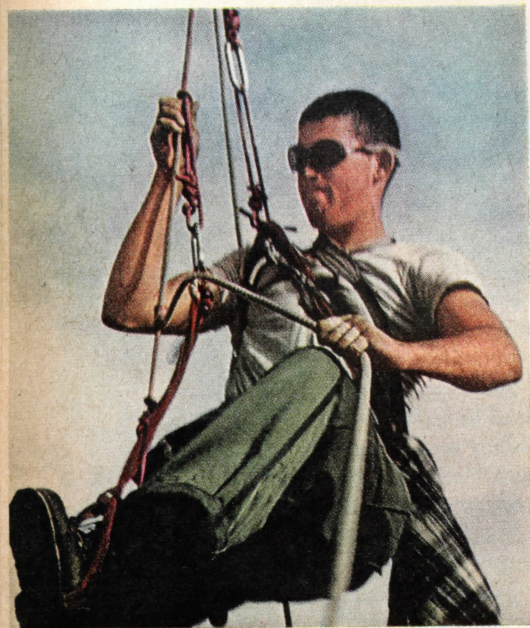
After manila rope broke under climber's weight, crew tested all-new nylon gear.
